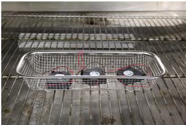
Photograph A-2: Test setup, samples inside conditioning chamber
