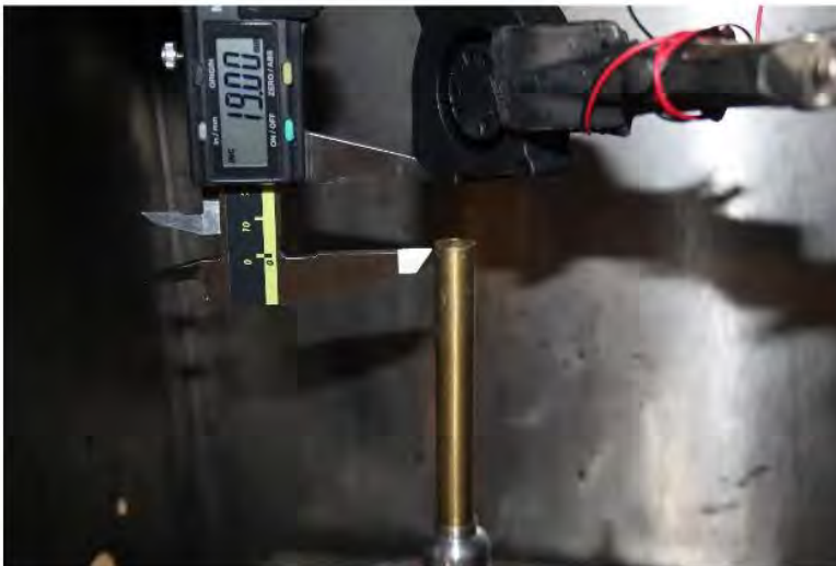
Photograph A-6: Representative Test setup, sample distance to burner
