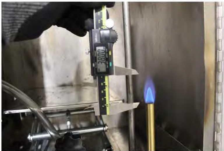
Photograph A-4: Outer flame height verification
