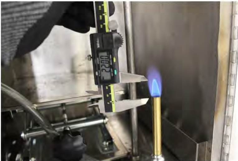
Photograph A-5: Inner flame height verification
