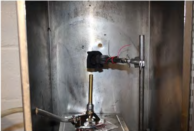
Photograph A-7: Representative Test setup, Vertical Burn
