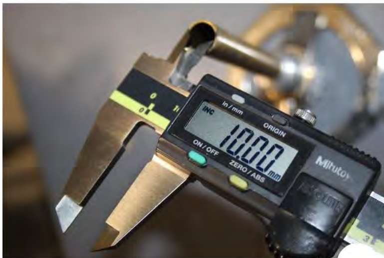
Photograph A-3: Bunsen burner inner diameter verification
