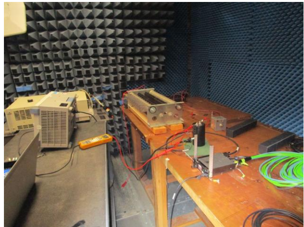
Section 16 Category B Setup with 10000uF Capacitor
