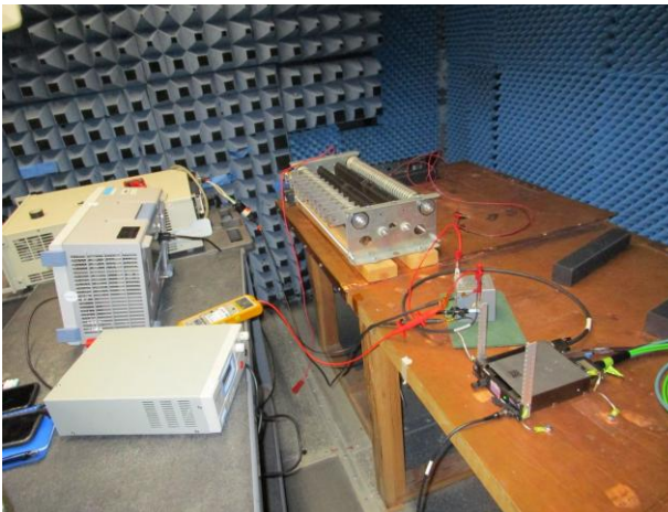
Section 16 Category B Setup with 10uF Capacitor
