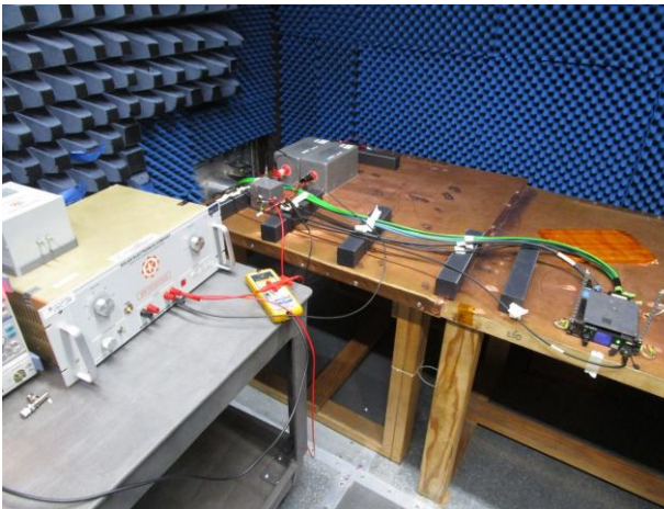
Section 17 Voltage Spike Test
