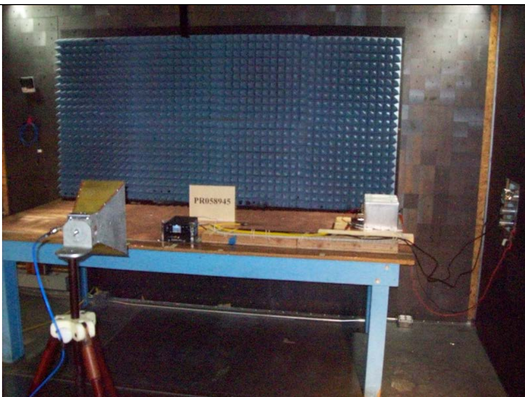
Photo 9. RE102 Test Setup. 1000 – 6000 MHz Horizontal
