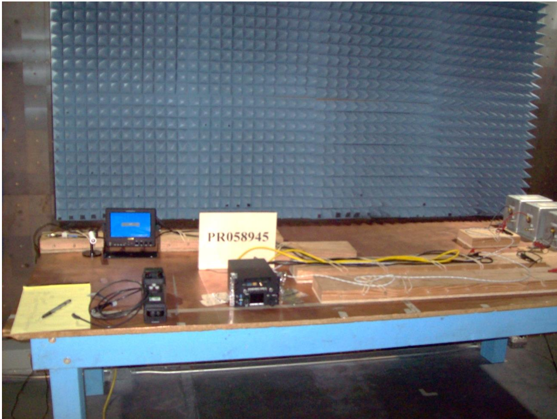
Photo 1. Electrostatic Discharge Test Setup.
