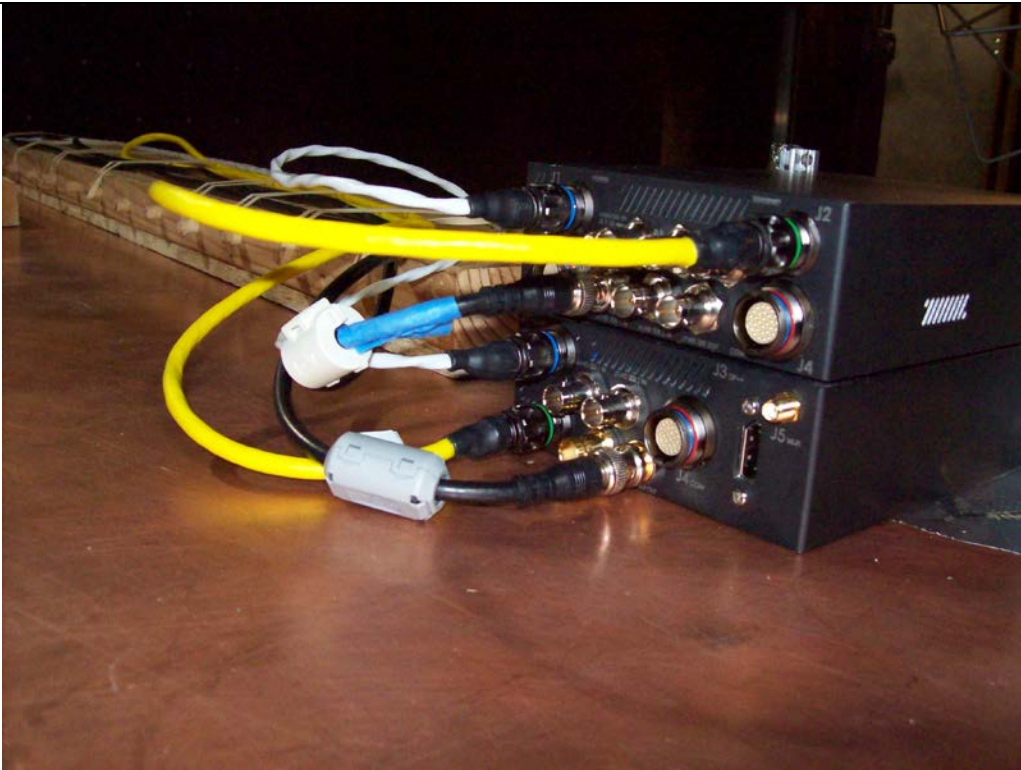
Photo 10. RE102 Test Setup. Ferrite installed on video cables
